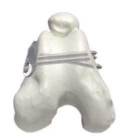
Screw orientations were evaluated and the trajectories of the distal screws were established in order to eliminate any possible violation of the joint space and any interferences with the trochlear ridge.
